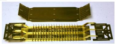
Bend the Top Frame Sheet over the ends of the Keel ensuring the tabs on the Keel engage the slots on the ends of the Top Sheet. Repeat for the opposite end.
